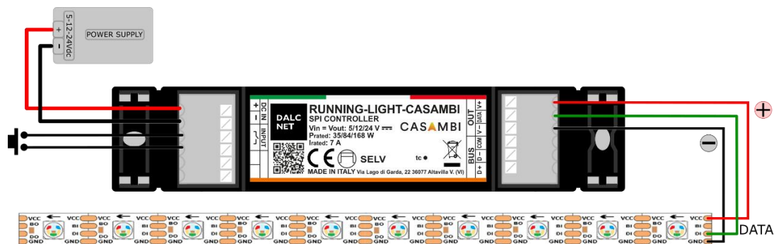
Figure 2: Connection diagram for Digital LED loads
